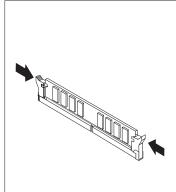
Figure 12. Installing the memory module
